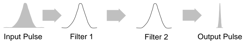
Figure 335. Effect of Multiple Filters on Signal Pulse
